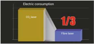
Amada's fibre laser has a higher energy conversion and 3 times higher energy efficiency than a  $\rm CO_2$  laser. Power consumption of the oscillator is also substantially reduced. There is no need for warm-up operations or laser gas, providing a running cost saving of at least 70%.
